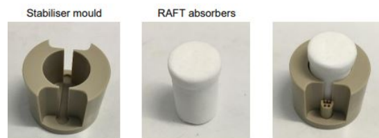
Figure 2.9: Manufacturing equipment for EngNT with the tethered PC method (extracted from [16])
