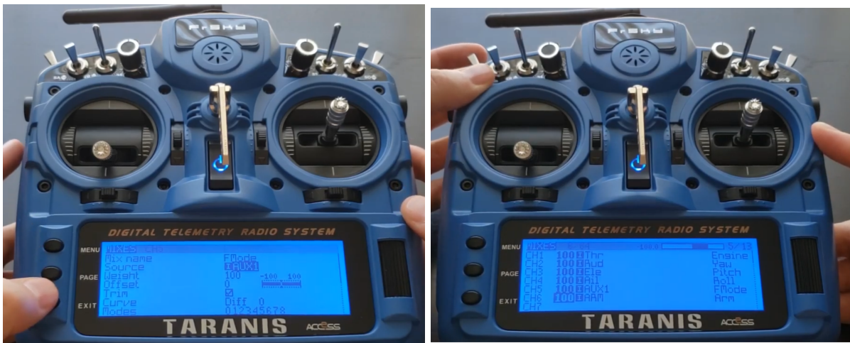
Figure 51: mapping each physical input of the remote to a different radio channel. Sources: https://www.youtube.com/watch?v=w40P1CQQ9Ls
