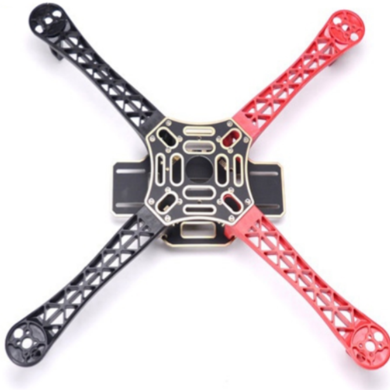
Figure 2: Typical frame of a drone: it is composed of a top plate, a bottom plate and independent arms. Sources: https://tinyurl.com/44vu2z68
