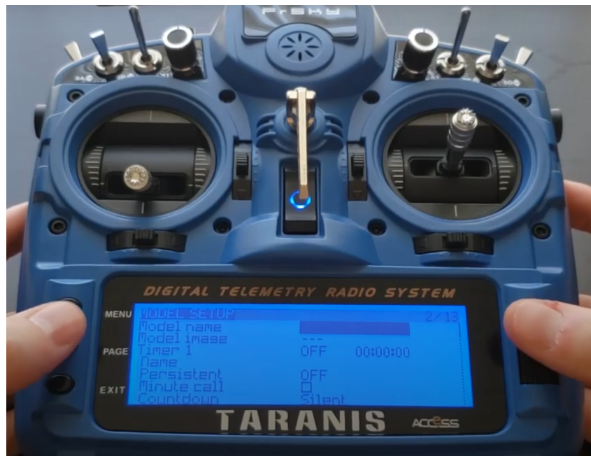
Figure 49: Creation of a new model in the remote, to store future parameters.
