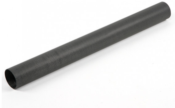
Figure 63: Carbon fiber tube used to make the arms of the drone. They will have to fit into the other parts.
