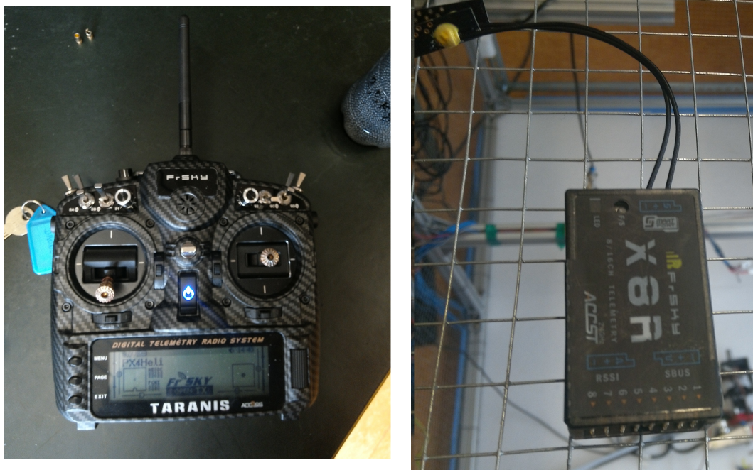
Figure 35: The Tanaris x9 remote control on the left, the FrSky X8R receiver on the right, used in combination of the kit.
