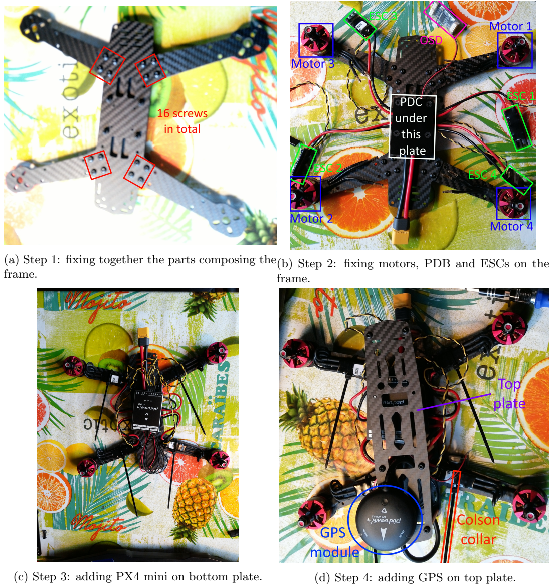
Figure 36: The different steps of the kit assembly.
