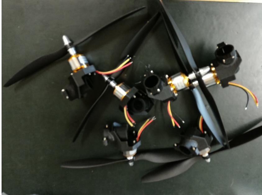
Figure 71: The first step of the assembly: fixing motors on motors mounting.
