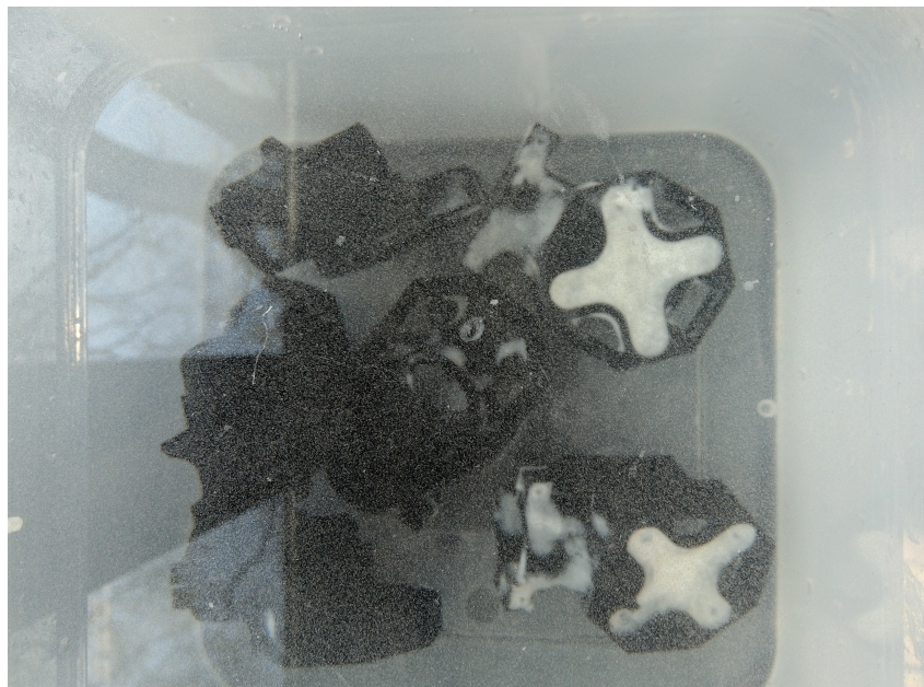
Figure 70: Motor mounting immersed in water to remove the support at the central tube.
