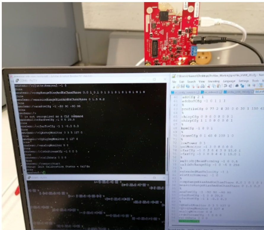
Figure 4.4: Successful device programming using PuTTY terminal emulator.
