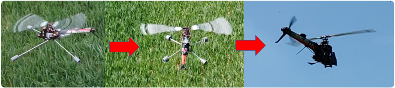
Figure 5.1: Evolution of the training kit feet length along the flight tests.
