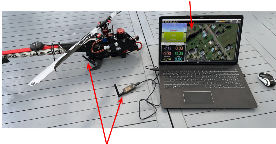
Figure 3.2: Telemetry modules connecting the flight controller to the ground control station.
