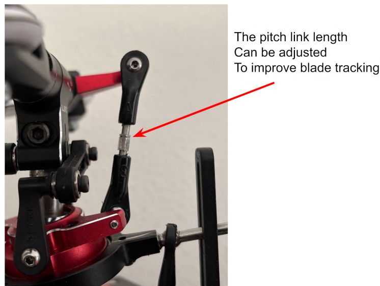
Figure 6.3: Pitch link of the Devil 380 with adaptable length.
