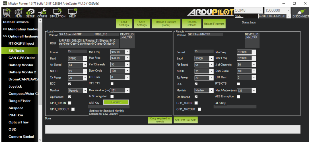
Figure C.2: Telemetry module binding page on Mission Planner.
