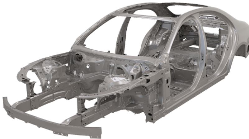
Figure 1.2: 3D scan of the full Mercedes S Class chassis by A2Mac1
