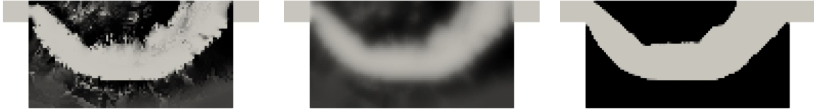
(a) Design field \alpha . (b) Regularised design field \tilde{\alpha} . (c) Regularised and projected field \beta .
