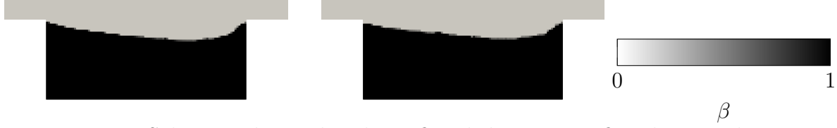
Figure 3.16: Solutions obtained with topO and dynamicTopO with a marching step coefficient of 1 for R = 10 mm; \omega_{Pt} = \omega_{th} = 0.5 .
