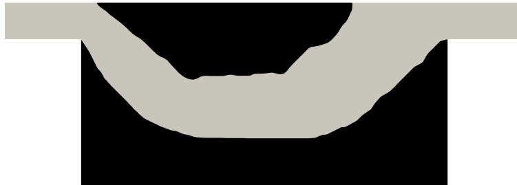
Figure 3.22: Topology of the domain in which the body-fitted validation will be done; solid material in black with real solid boundaries.
