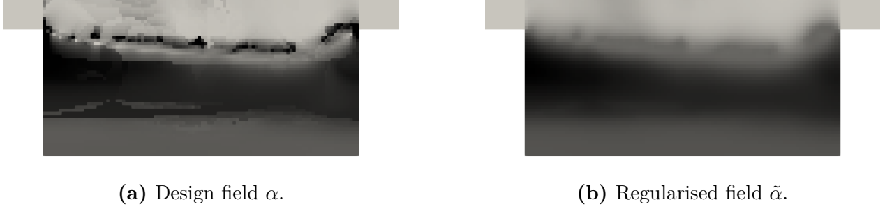
Figure 2.7: Design field \alpha and the regularised field \tilde{\alpha} of a solution with a big regularisation radius.
