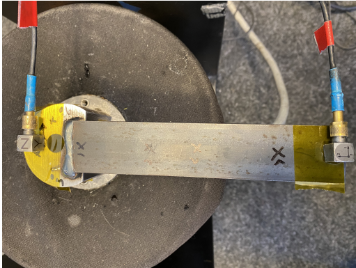
Figure 4.11: Sine sweep test in open loop on the VTS VG-100 shaker with a beam structure.
