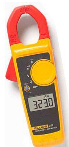
Figure 3.14: Measurement of the current signal with a current-clamp.
