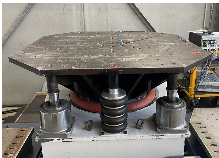
Figure 4.46: Load support guidance of the expander on the 120-kN shaker.
