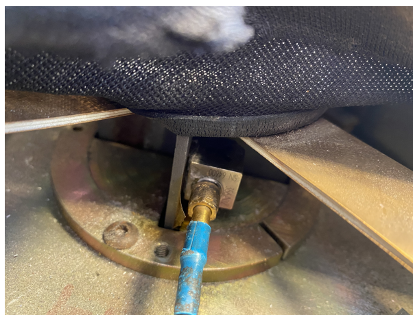
Figure 3.9: Accelerometer placed near the coil of the VTS VG-100 shaker.
