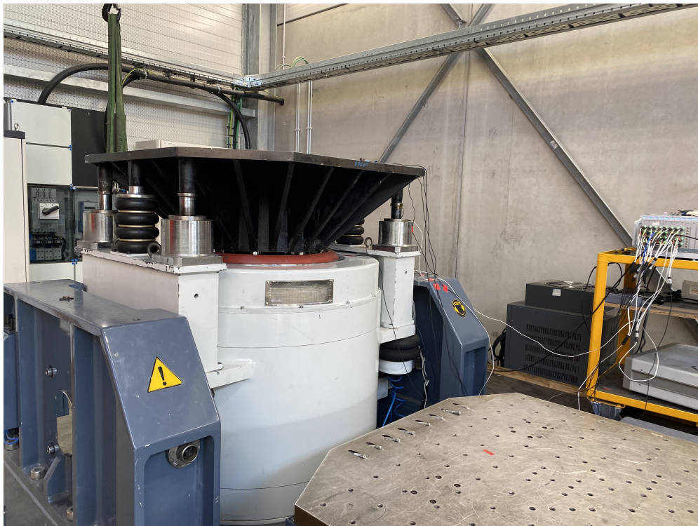
Figure 3: Studied shaker for the more advanced tests: 120-kN DongLing shaker.
