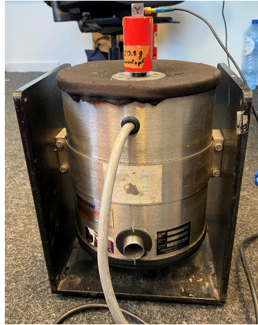
Figure 2: Studied shaker for the preliminary tests: VTS VG-100.
