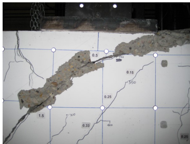
Figure 4.53: Shear-induced flexural crushing in specimen C2N (courtesy by Andermatt and Lubell, University of Alberta)
