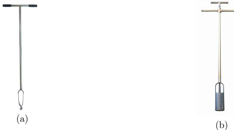
Figure 2.7: Soil sampling equipment with (a) the auger and (b) the root auger. *Source: Eijkelkamp*
