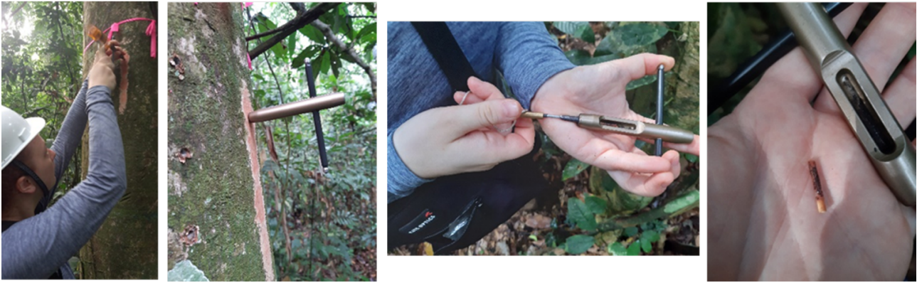
Figure 1.3: Micro-coring process. From the left to the right: (i) insertion of trephor with a hammer (ii) inserted micro-core ready for extraction (iii) extracting the micro-core from the trephor device (iv) trephor with micro-core showing the xylem (white tissue) and bark (darker tissue) from a Panda oleosa tree.
