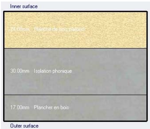
Figure 50 : DesignBuilder - Construction – Sol intérieur - Illustration
