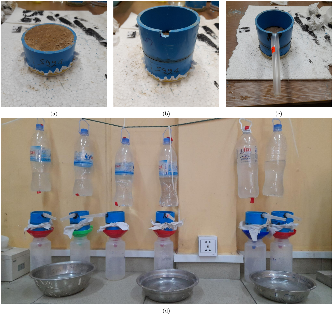
Figure 20: Handcrafted conductivity at saturation device. (a) sample ring, (b) constant head ring stick with a silicon joint, (c) excess water discharge spout, (d) final device with control overflow drip system to maintain a water constant head
