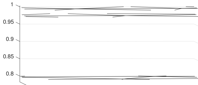
(b) Slice of the model with only horizontal edges of the finite elements represented, to show the three individually meshed layers of different thicknesses
