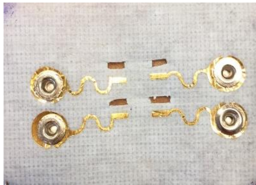
Figure II.7: Gold electrodes on a PET substrate embedded into medical tape (from [41])
