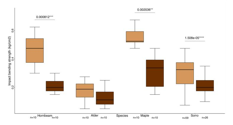
Figure 27: Boxplots of the impact of species and treatment on the impact bending strength (kg/cm2). Wilcoxon test is used to compare the species/treatment. The p-value is added if there is a significant difference between two boxplots with the degree of significance.
