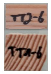
Figure 16: Difference between an L, R, T sample (top picture) and an R, T, L sample (bottom picture)
