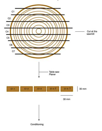
*Figure 12: Cutting scheme of temperate species before conditioning*
