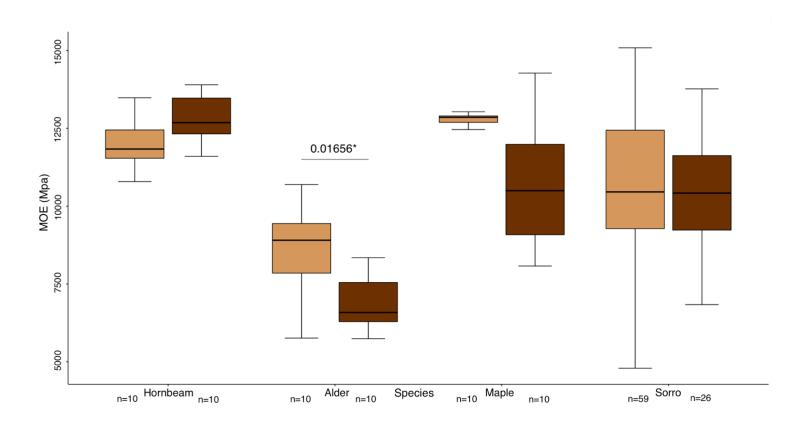
Figure 25 : Boxplots of the impact of species and treatment on modulus of elasticity (MPa). Wilcoxon test is used to compare the species/treatment. The p-value is added if there is a significant difference between two boxplots with the degree of significance
