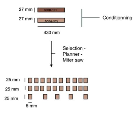
Figure 15: durability samples preparation
