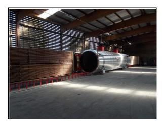
Figure 9: Maspel oven Model TVS 6000 WDE Maspell srl, Terni, Italy) at Scidus company, Etalle, Belgium.
