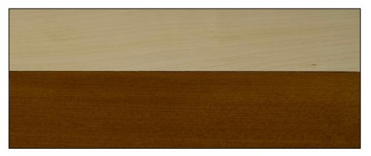
Figure 4 : Color difference between (a) untreated and (b) heat treated Acer pseudoplatanus
