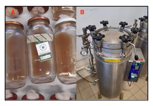
*Figure 18: autoclave process. A: control label to prove that the samples have been autoclaved. B: autoclave system*
