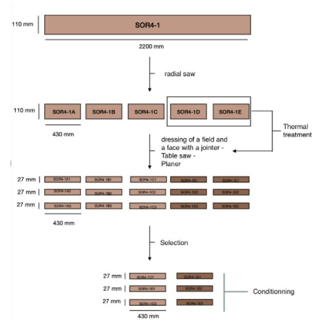
Figure 10: Cutting scheme for the physico-mechanical tests before conditioning
