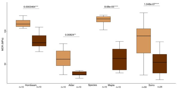
Figure 26 : Boxplots of the impact of species and treatment on the modulus of rupture (MPa). Wilcoxon test is used to compare the species/treatment. The p-value is added if there is a significant difference between two boxplots with the degree of significance.
