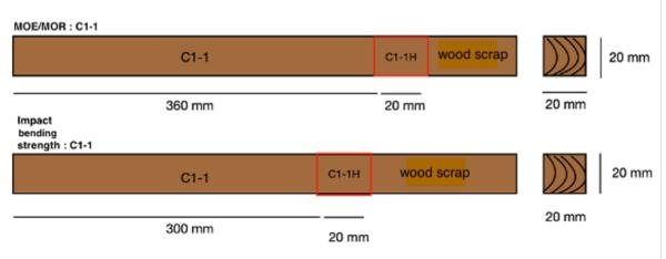
Figure 13: Cutting scheme for MOE/MOR and impact bending strength tests and humidity samples (H)
