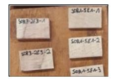
Figure 14: samples for durability tests (fungi and termites)
