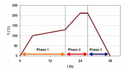
*Figure 3: Evolution of the temperature over time for a thermal treatment. Source: http://www.heatwood.se/*
