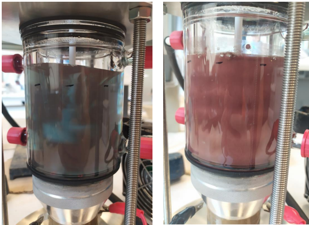
Figure 46 Photos of US assay 91, taken 5 and 30 minutes into the reaction (left and right image, respectively). Copper particles make the solution opaque. On the right, crests and troughs of the modulated wave signal are seen
