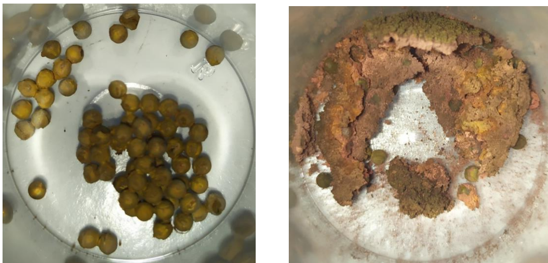
Figure 36 Left, solid residue from assay 8 obtained after filtration (fine residue was separated). The beads are strongly stuck together in the shape formed at the bottom of the reactor; Right, solid residue from assay 93
