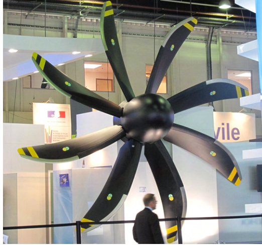
Figure 1.3: Airbus A400m propeller blades in Paris Airshow, 2009
