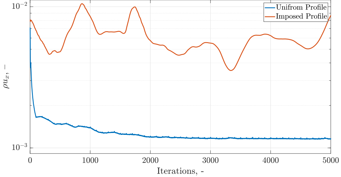
Figure 4.3: Mean Navier-Stokes residual of \rho u_x for high crosswind with uniform and imposed BL profile at inlet.
