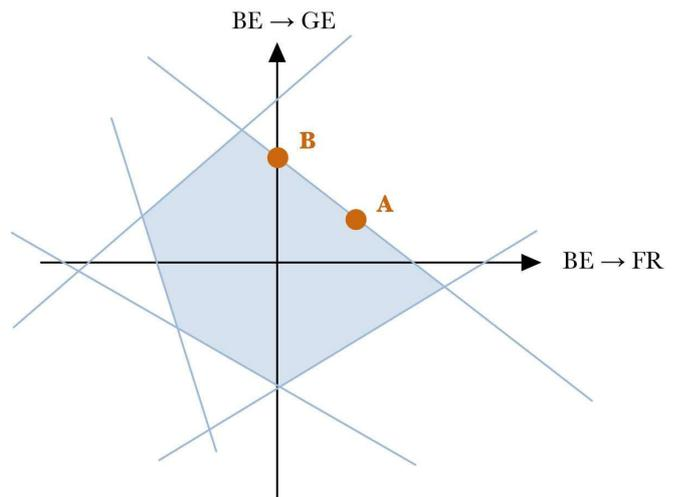
Figure 20: 2D example of a FB capacity domain
