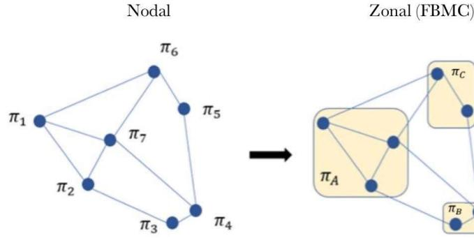
Figure 10: In the FBMC method, only one equivalent node per zone is considered, but all critical lines are taken into account
