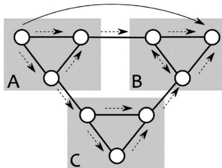
*Figure 8: A commercial transaction between zone A and B causes physical flows through other parts of the grid.
