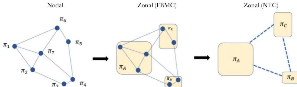
Figure 6: Illustration of zonal aggregation of injection points
