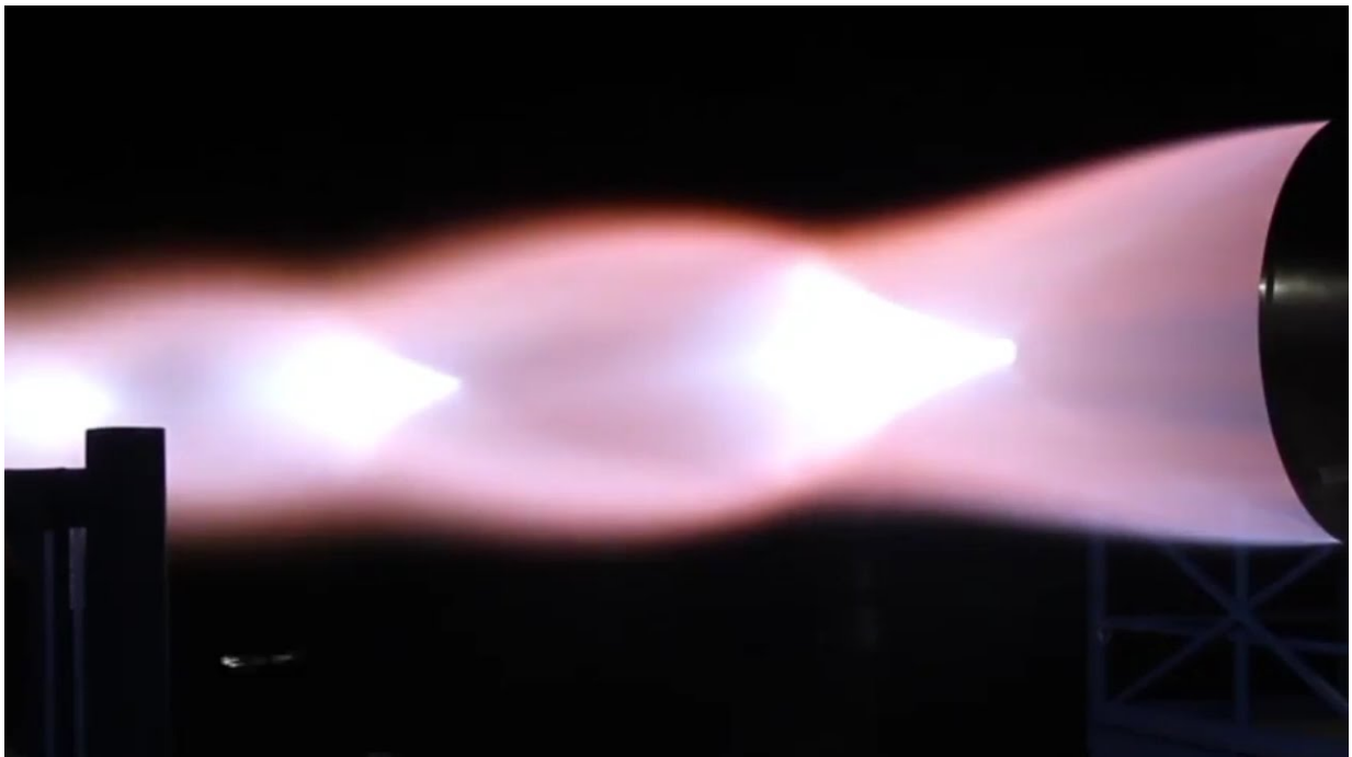
Figure 2.4: Overexpanded jet during a SpaceX Raptor Engine Test
