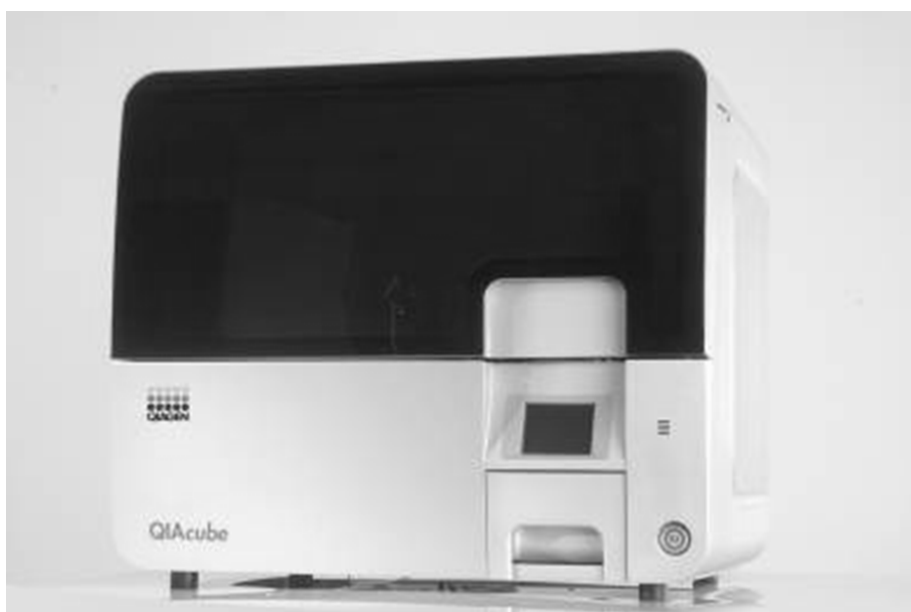
Figure 1. Automated DNA purification. DNA purification using the QIAamp Fast DNA Stool Mini Kit can be automated on the QIAcube.
