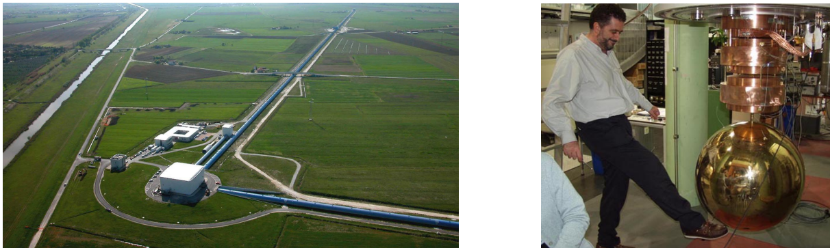
Figure 6: From [30] and [31]. On the left it is an aerial view of the Virgo interferometer located at Cascina near Pisa in Italy. Its arms are 3 km long and the detector operates at frequencies between 20 Hz and 1 kHz. It became operational in 2007. On the right, we have the resonant antenna MiniGRAIL at Leiden University in the Netherlands. Its spherical design allows equal sensitivity in all directions, with a resonant frequency of 2.9 kHz.
