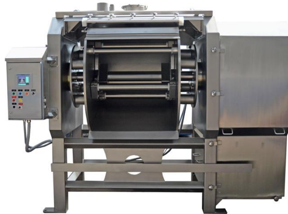
Figure 6 : Mixer horizontal (Open frame tree-roller bar horizontal mixer). 1
