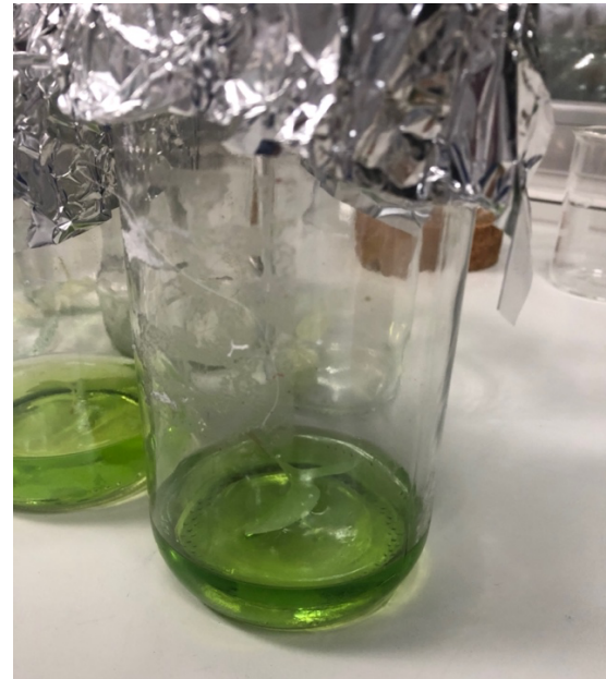
Appendix 15. Aerial part of the pepper plants macerating in methanol, after the experiment, for the metabolites' extraction.
