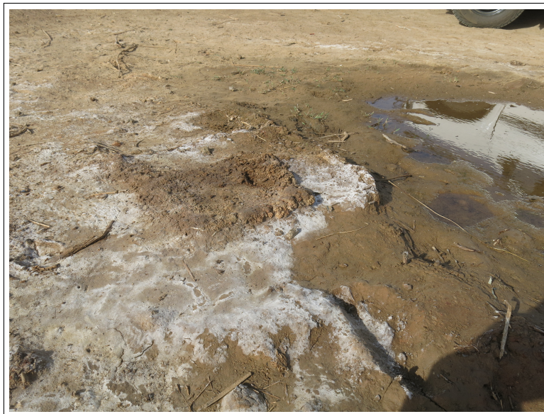
Figure 15: Salt precipitation observed at the surface near the KN4 piezometer, along the Gorom Upstream distributary.
