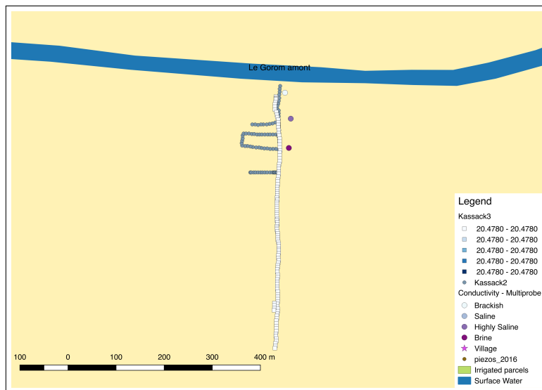
Figure 65: Geographical representation of the EM profile at Kassack (split into two data sets). The entire dataset measured a conductivity of 20.5 mS/cm.
