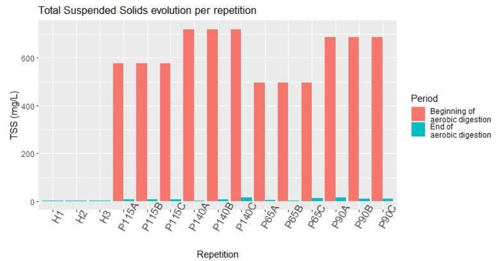
Figure 3.12: Comparison of pH, BOD5, COD and TSS between the beginning and the end of the aerobic digestion phase per repetition
