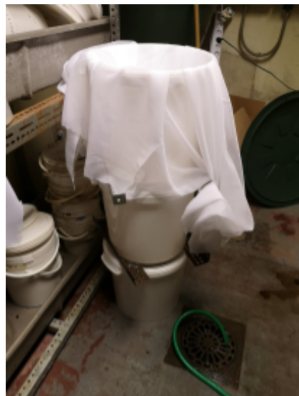
Figure 2.3: The filtering system used after the anaerobic digestion phase
