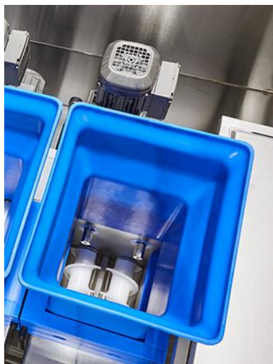
Figure 97 : Cuve d'extrusion ( https://www.readingbakery.com/low-pressure-extruder-bakery-equipment.html ).
