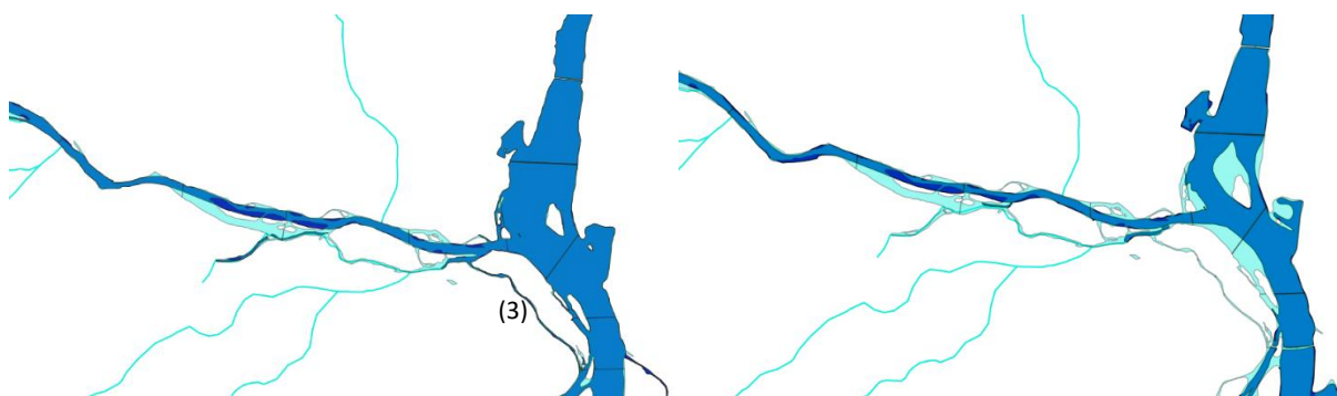
Figure 28: Representations of the changes in the shape of the river Gausa at its confluence with Gudbrandalslagen between 1947 (light blue) and 1959 (dark blue) on the left and 2019 on the right (dark blue)
