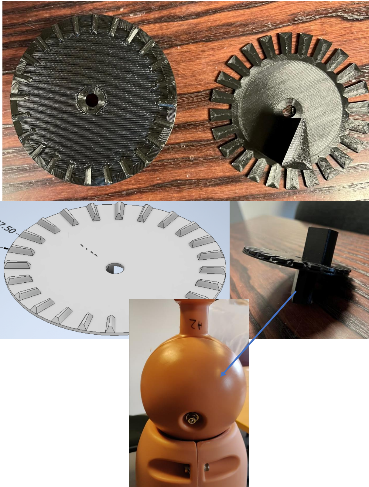
Figure 66 - Parts added to the ball joints to fix them
