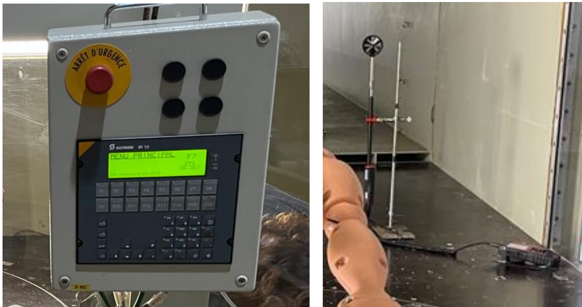
Figure 69 - Control box (left) and anemometer (right)
