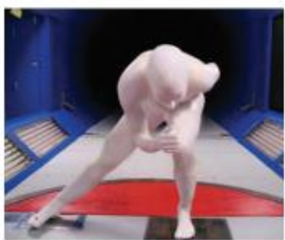
Figure 9 –Sidepush position in the test section (D'Auteuil et al., 2012)
