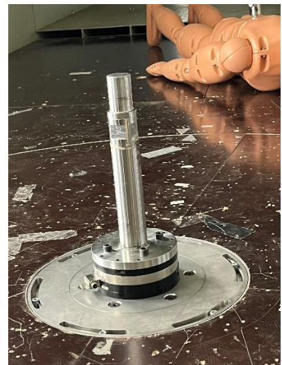
Figure 68 – Wind tunnel of the university of Liège, and the aerodynamic balance on which the model will be pose
