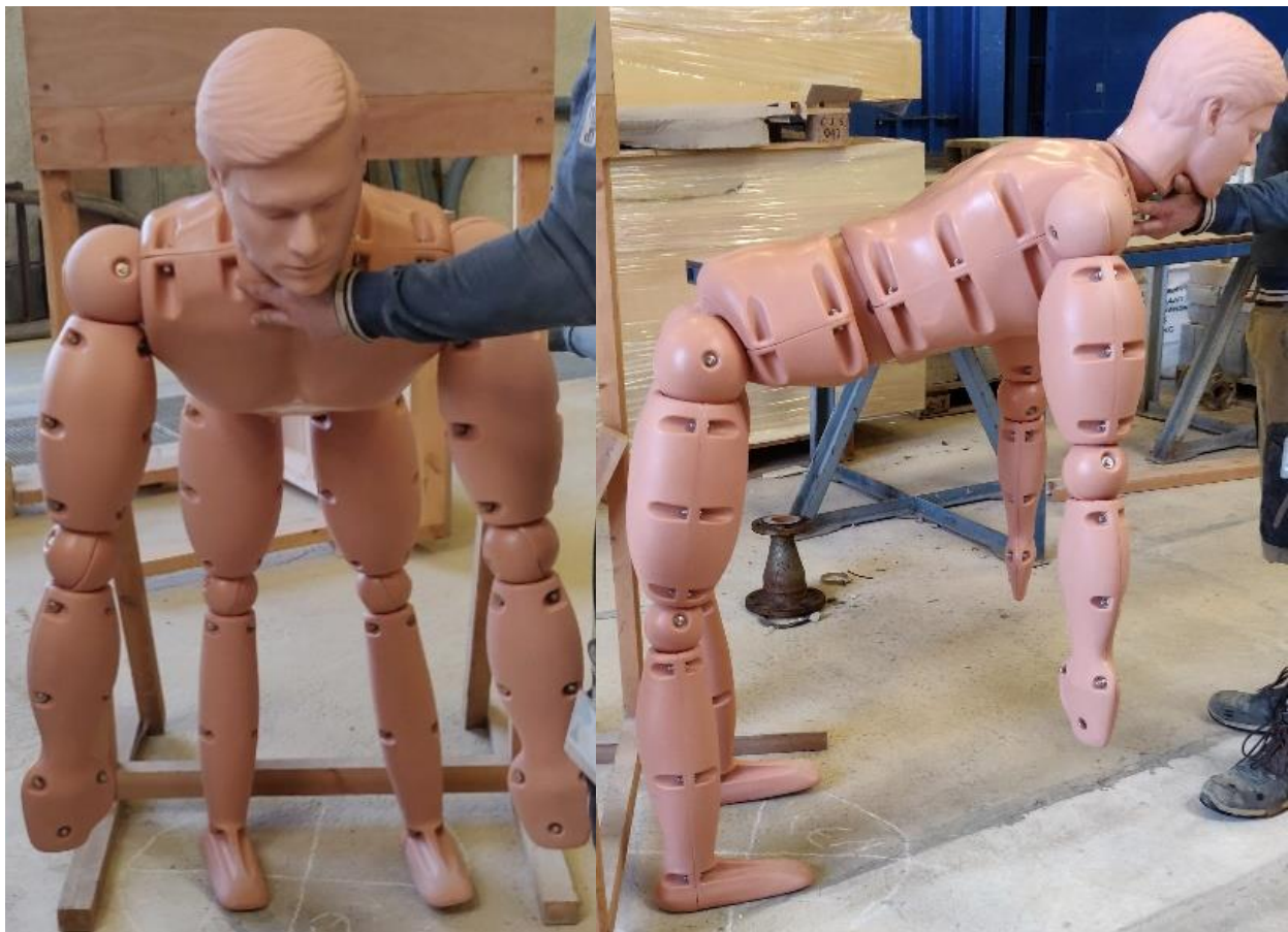
Figure 3 - Picture of the reference position of a model: front and profile view
