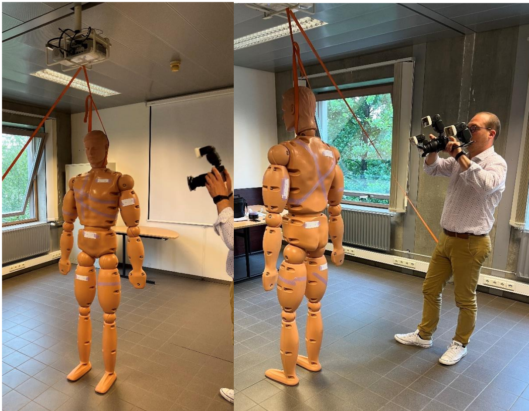
Figure 51 - Data acquisition of the model using a three flashes camera with polarizer
