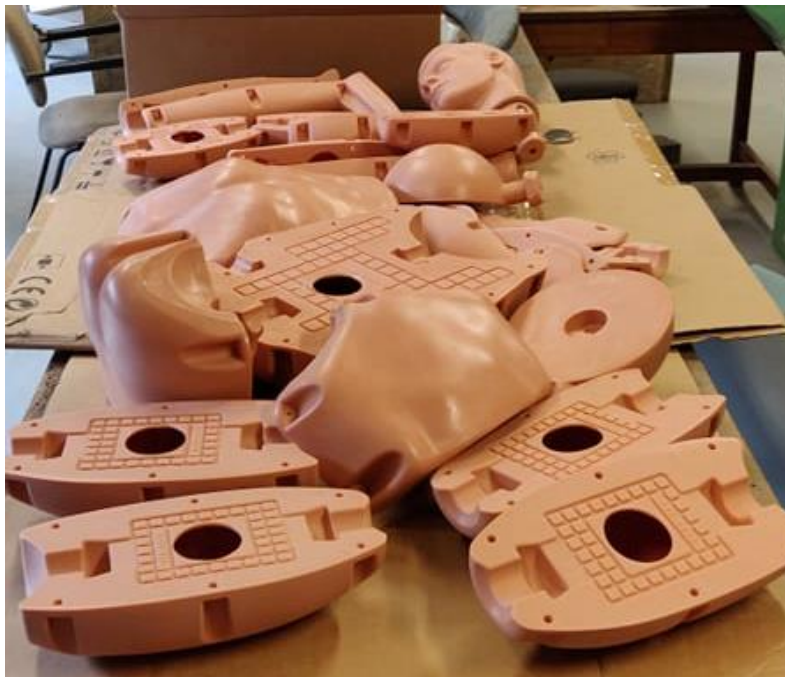
Figure 14 - Picture of Ken disassembled, where the holes which allow to fill Ken are visible
