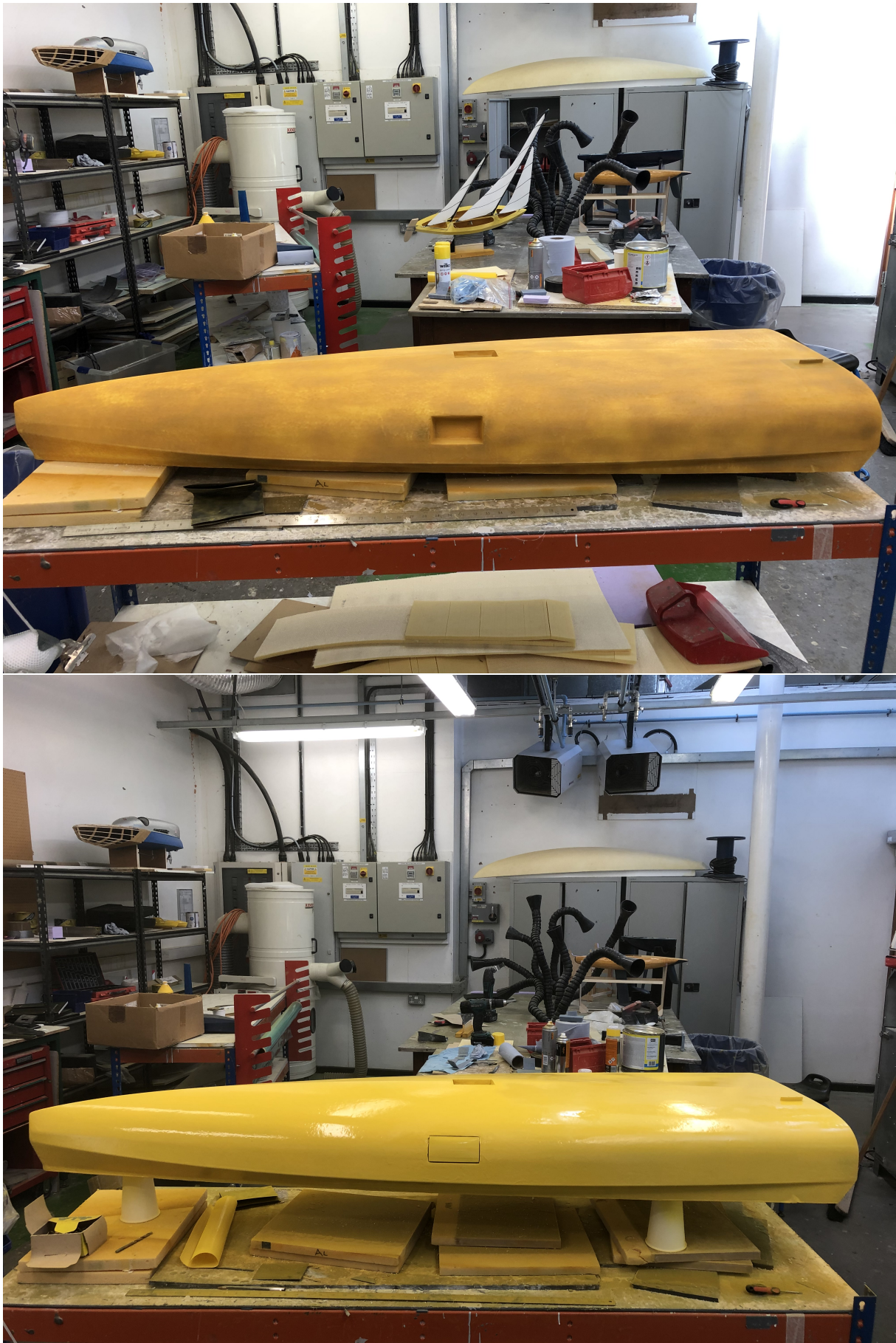
Figure 56: Primer and paint application on the hull
