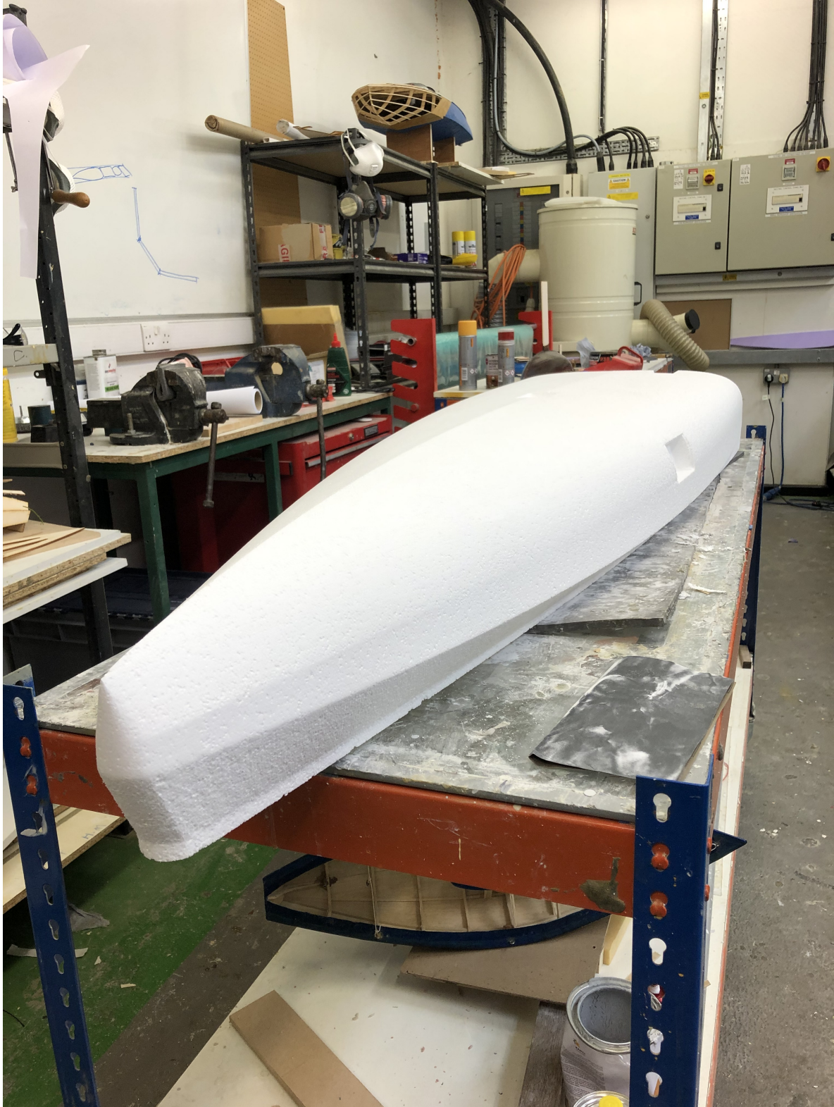
Figure 54: CNC milled polystyrene hull
