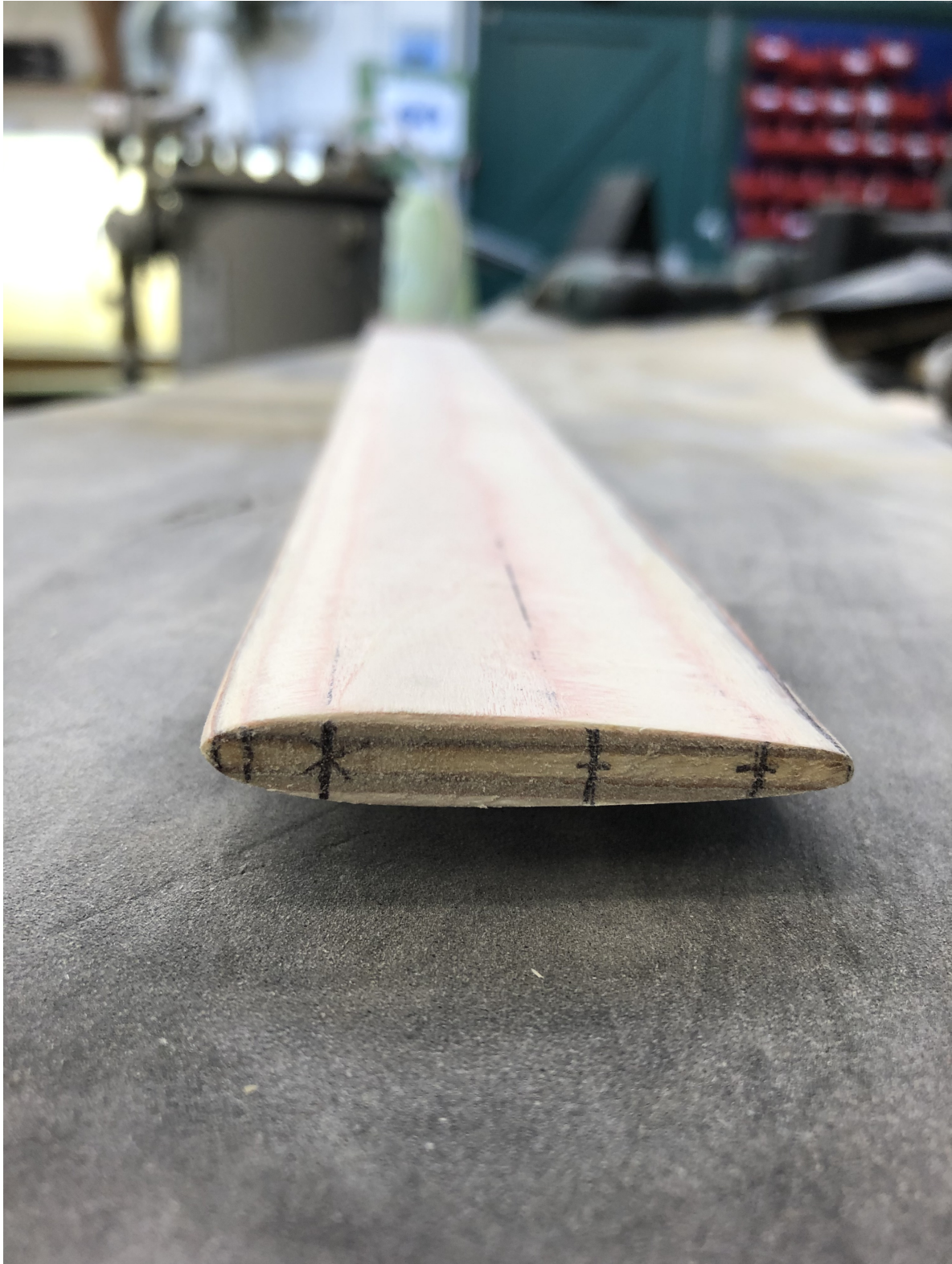
Figure 59: New keel shaped in plywood
