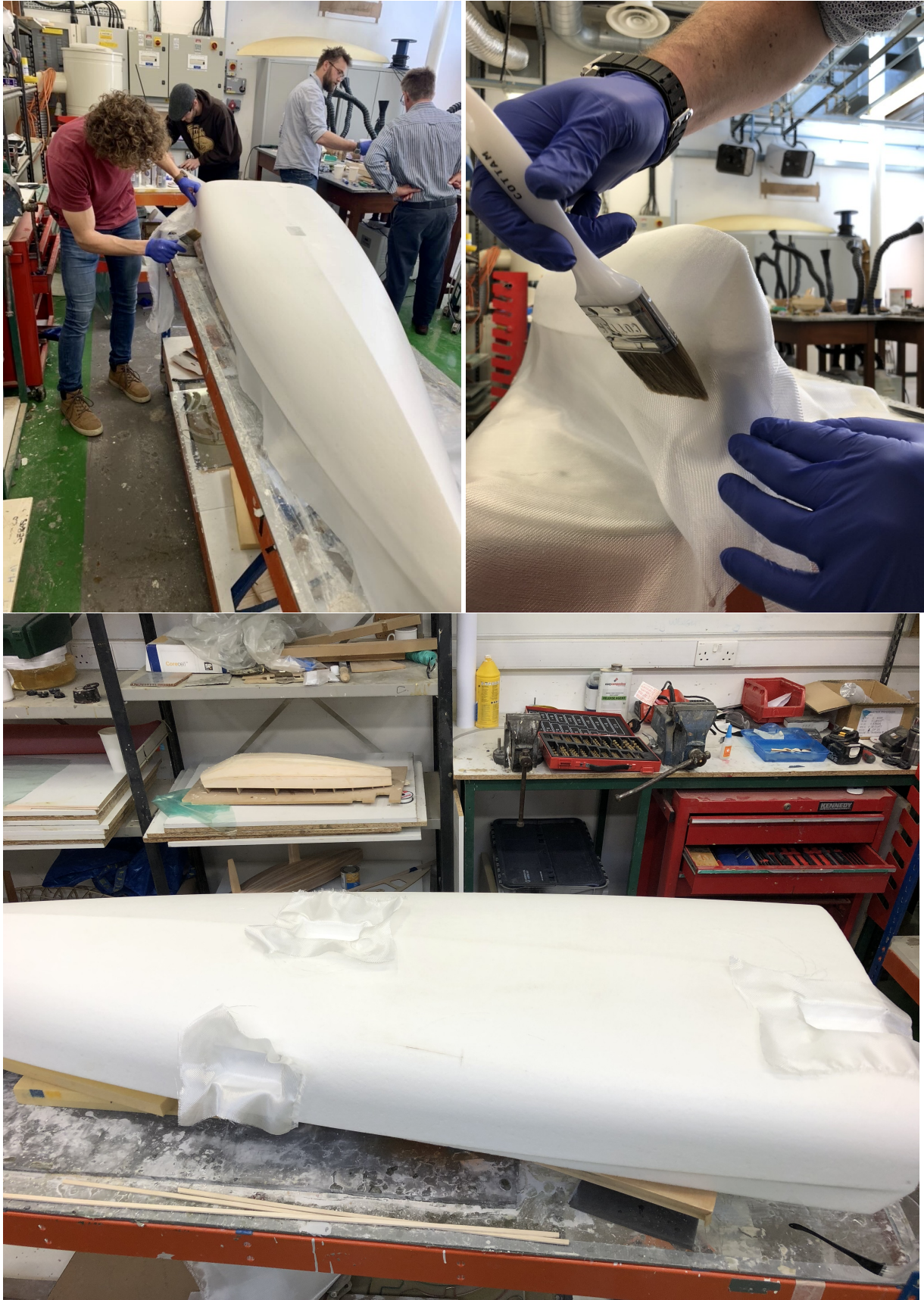
Figure 55: Glass fiber application on the hull
