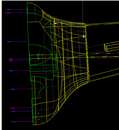
Figure 3.26: Boundary conditions used to simulate the symmetry of the drone
