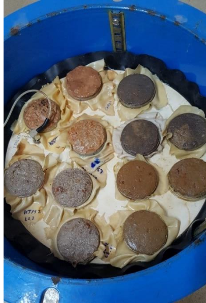
Figure 15 - Samples in the pressure plates
