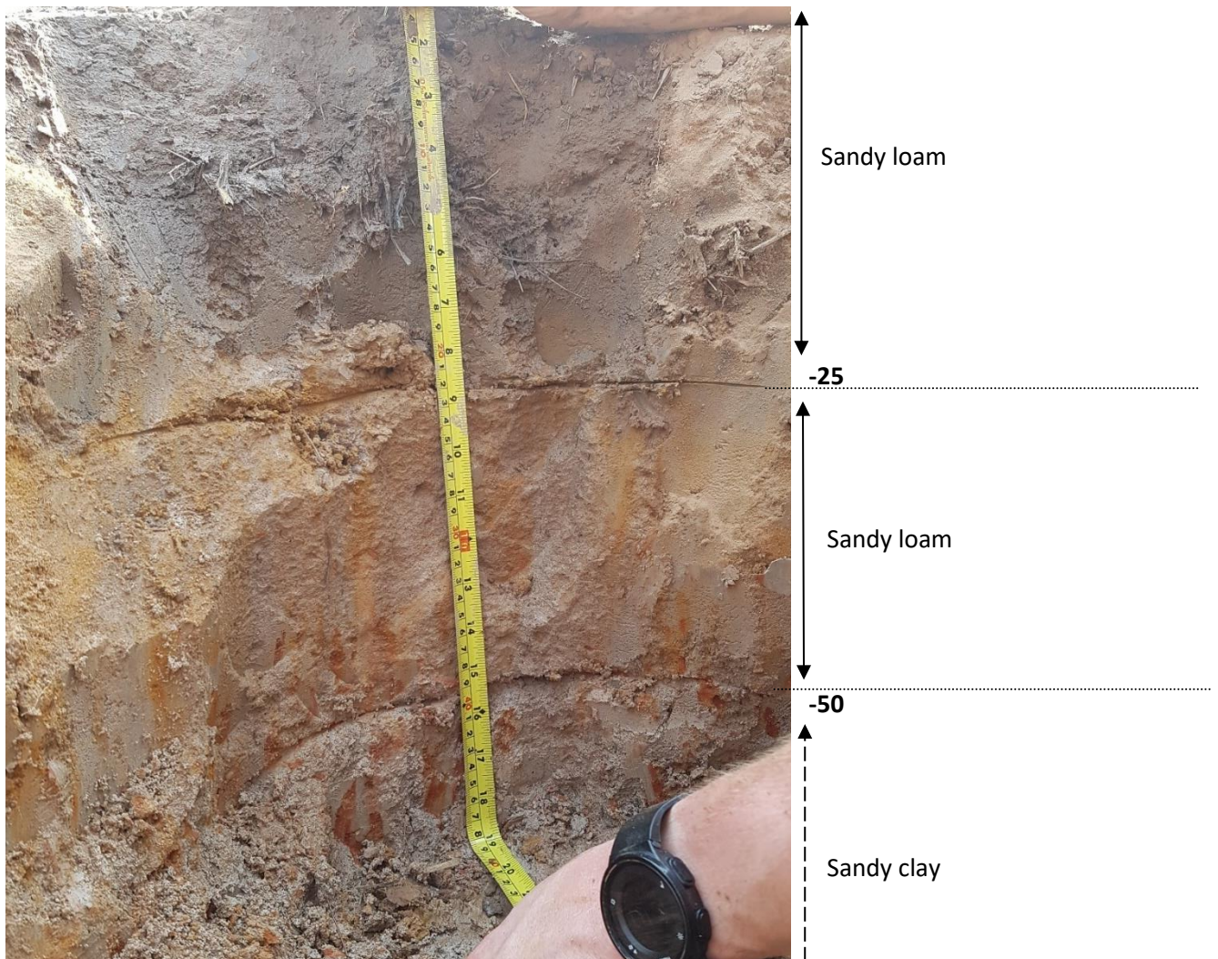
Figure 19 - Soil profile of the first experimental site in the Kampong Thom province (02/03/22)
