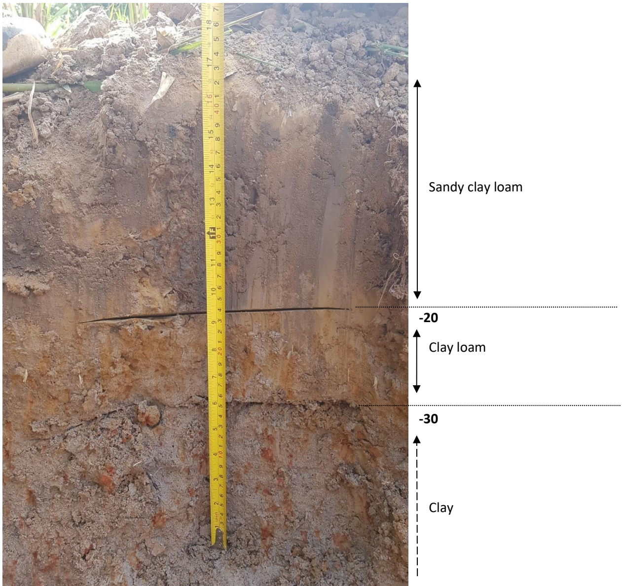
Figure 23 - Soil profile of the second experimental site in the Kampong Thom province (31/03/22)
