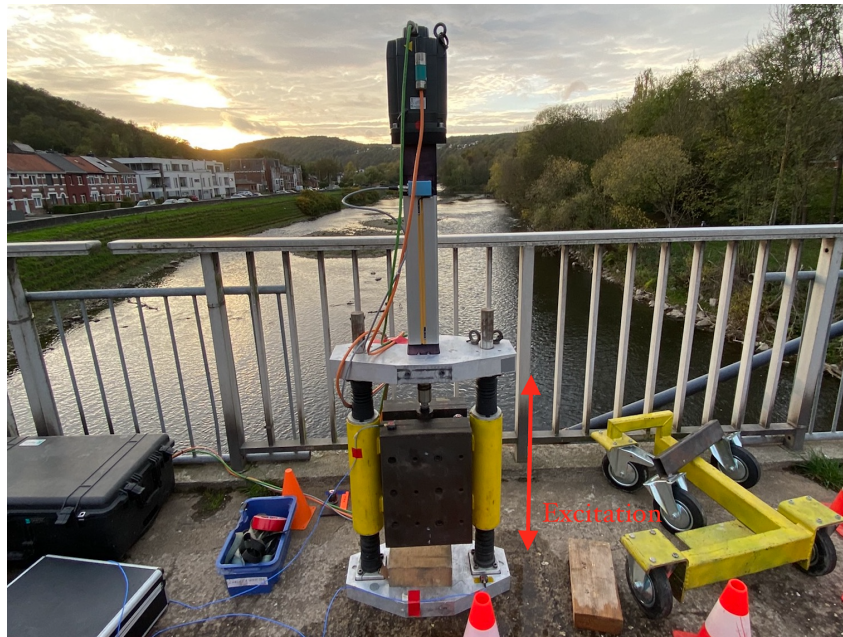
Figure 56: Picture of the shaker. The moving mass consists in the dark gray plates and the yellow cylinders attached to the linear actuators.
