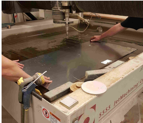
(a) Water jet cutter: Placing work piece on pool's grill
