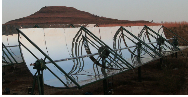
Figure 2.2: STG's parabolic trough collectors, installed in Lesotho [3]
