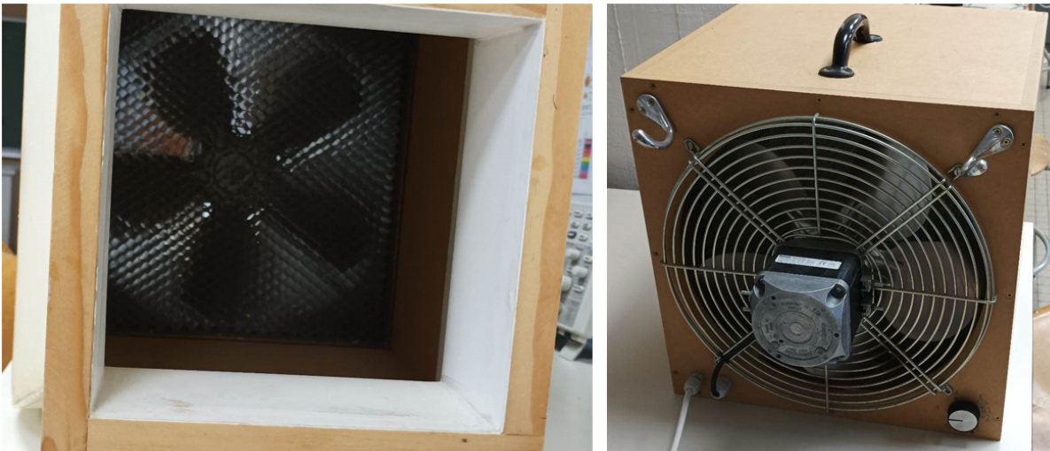
FIGURE 23 – Tunnel de vent
