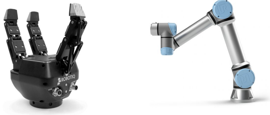
Figure A.1. (left) Three finger adaptive robot gripper from Robotiq. (right) The UR5.
