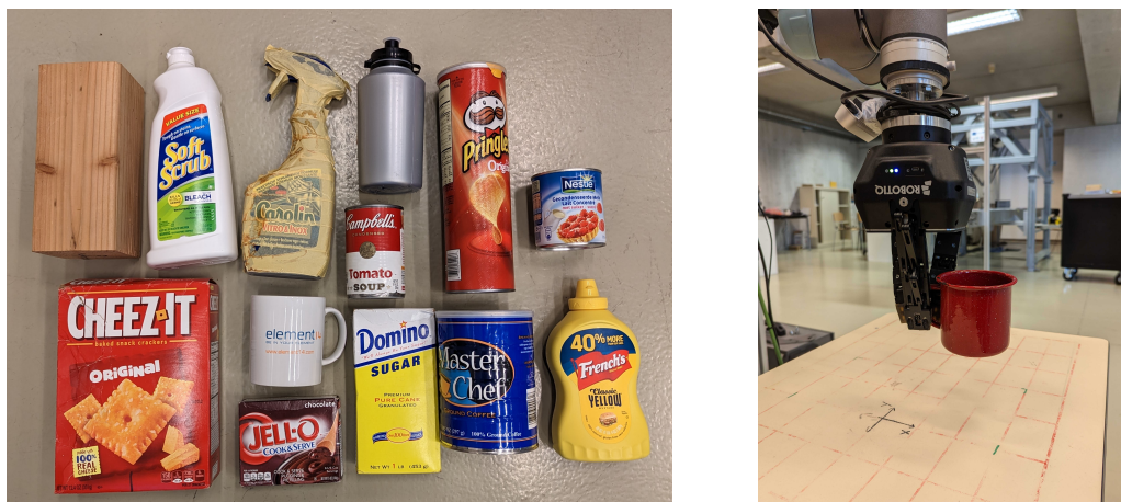
Figure 7.3. (left) Object assets used in the real setup. (right) Successful grasp of a mug.
