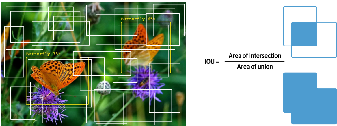
Figure 10: Illustration of a set of anchor boxes on the left and illustration of the Intersection Over Union on the right [21].
