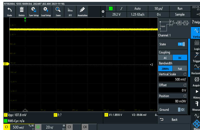
Figure 6.4: E-peas output voltage with no load.
