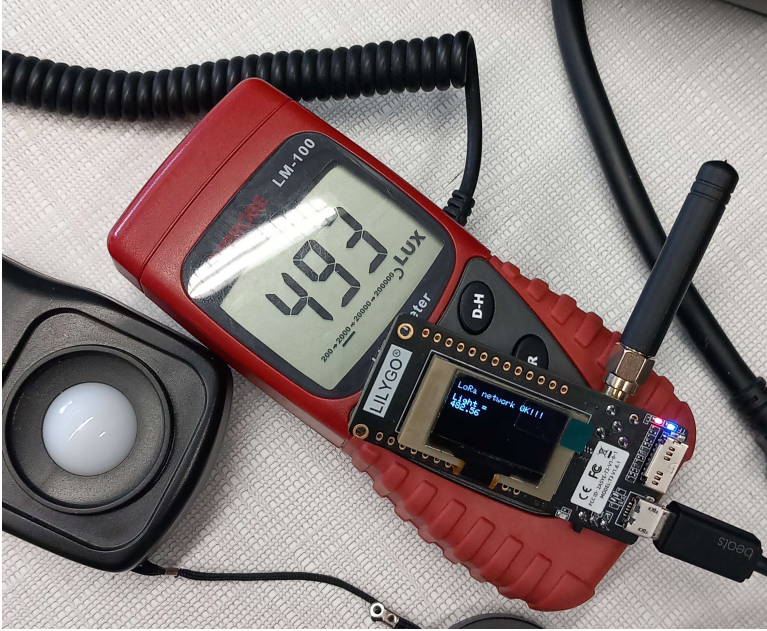
Figure 3.9: Comparison between the ambient light sensor and the lux meter (493 vs 482.56).
