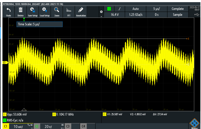
Figure 6.6: E-peas output voltage with a 120\ \Omega load (AC coupling mode).
