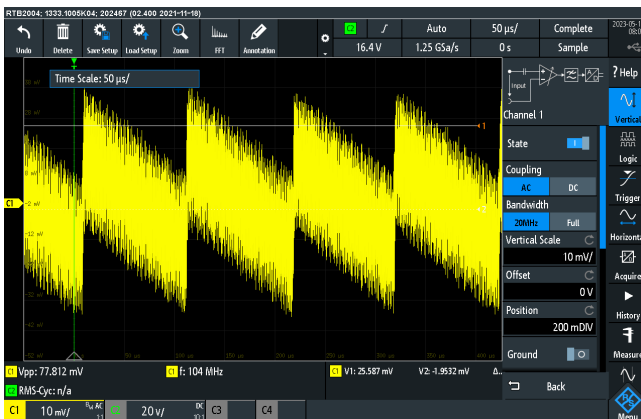
Figure 6.5: E-peas output voltage with a 1200\ \Omega load (AC coupling mode).
