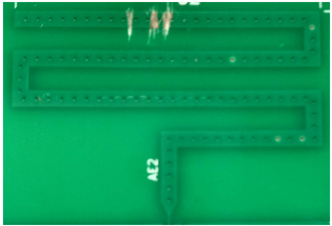
Figure 5.20: Practical meander antenna cut.
