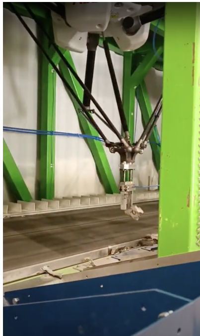
Figure 4.5.: Throw with the Flexpicker using TD3 algorithm.
