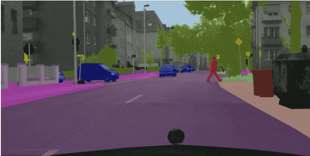
Figure 4.6. Segmentation mask from the Segformer architecture on the Cityscapes dataset. Segformer is able to recognize all the objects and regions in the image.
