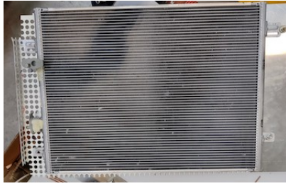
(a) External exchanger of the Renault ZOE (HTX1)
