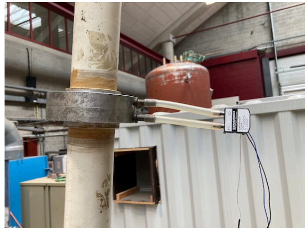
(b) Differential pressure sensor PDIFF500 (see Tab.2)
