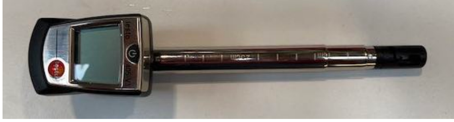
Figure 29: Anemometer used for the air flow rate measurement ( datasheet )
