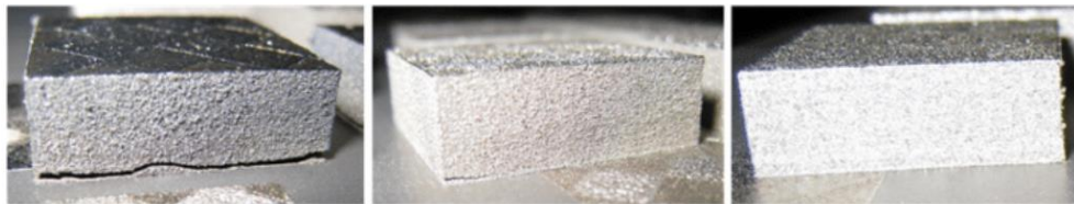
Figure 21. M2 HSS parts with preheating temperatures of 90°C (left), 150°C (middle) and 200°C (right) [85]
