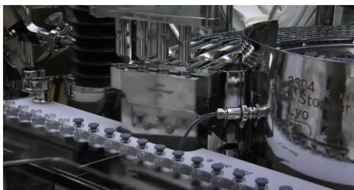
FIGURE 55 - COOK PHARMACICA 150 VPM FILLING LINE [89]
