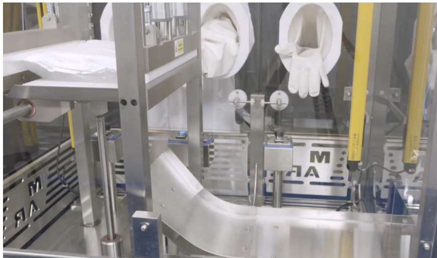
FIGURE 150 - MANUAL DE-BAGGING EXAMPLE
