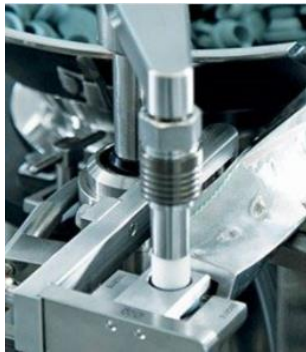
FIGURE 46 - FLEXICON FPC60 STOPPERING AXIS [82]
