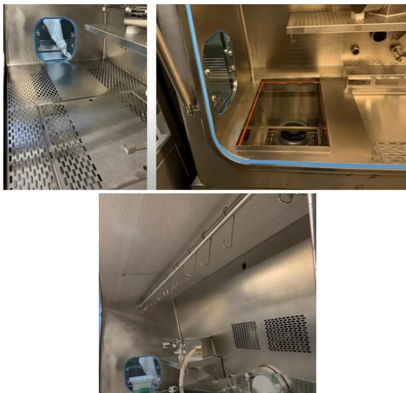
FIGURE 23 - INSIDE VIEW OF AN ISOLATOR [30]
