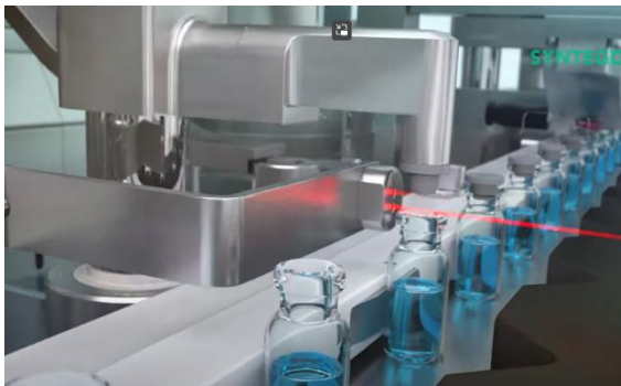
FIGURE 45 - VERSYNTA STOPPERING STATION [81]
