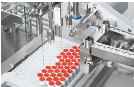
FIGURE 50- JEREMPLI NFL/1-2-RDL FILLING IN NEST STATION [85]
