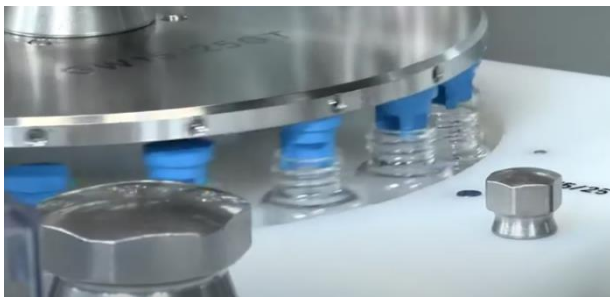
FIGURE 57 - BOSCH FLC 3080 STOPPERING STATION [90]
