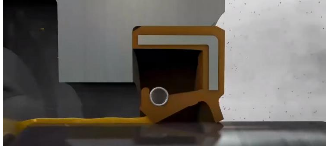
FIGURE 132 - FUNCTIONING OF A TC4 LIP SEAL [104]
