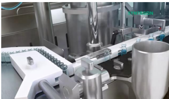
FIGURE 44 - VERSYNTA MACHINE ACHIEVING 30 VPM [81]
