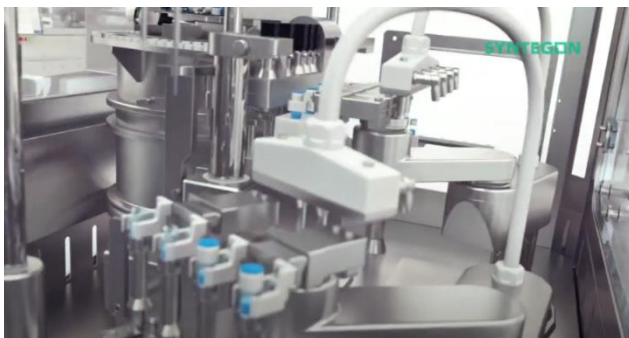
FIGURE 48 - VERSYNTA MACHINE ACHIEVING 60 VPM [83]
