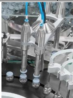
FIGURE 51 - SX-220-PP STOPPERING STATION [86]
