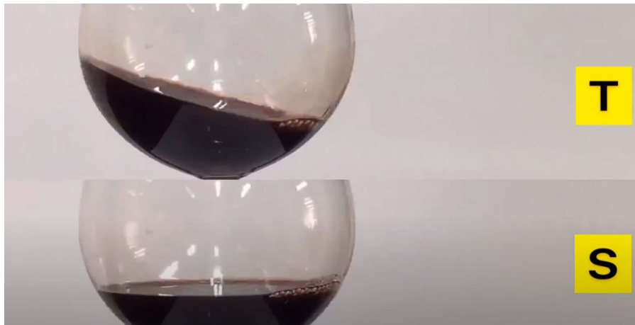
FIGURE 88 - IMPACT OF TRAPEZOIDAL AND S-CURVE VELOCITY PROFILE ON A GLASS OF WINE AT THE END OF THE MOTION [111]
