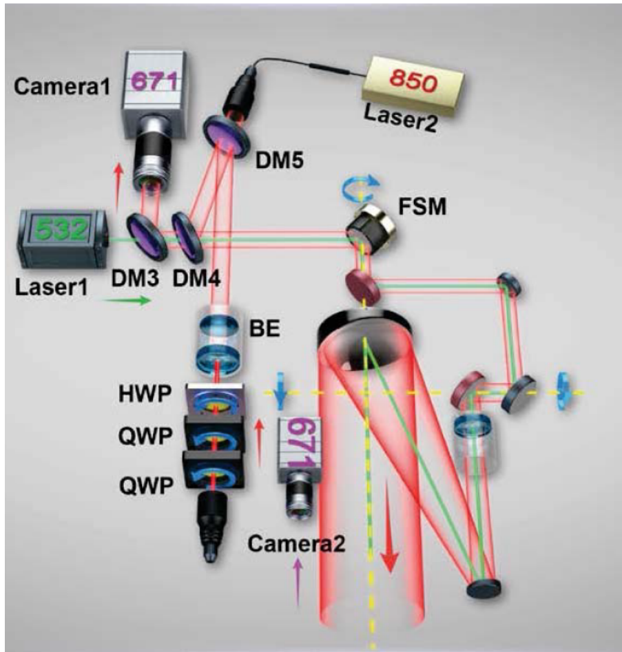
Figure 4.18: The signal beam passes through the motorised wave plates to correct the polarisation shift induced by the relative motion of the satellite. It is then expanded by a beam expander (BE) and combined with a pulsed laser at 850 nm for synchronisation and a green laser at 532 nm for tracking. The Fast Steering Mirror (FSM) is used for closed-loop tracking, based on the 671 nm beacon laser images captured by camera 1 and camera 2. Figure from Yin et al. [64].
