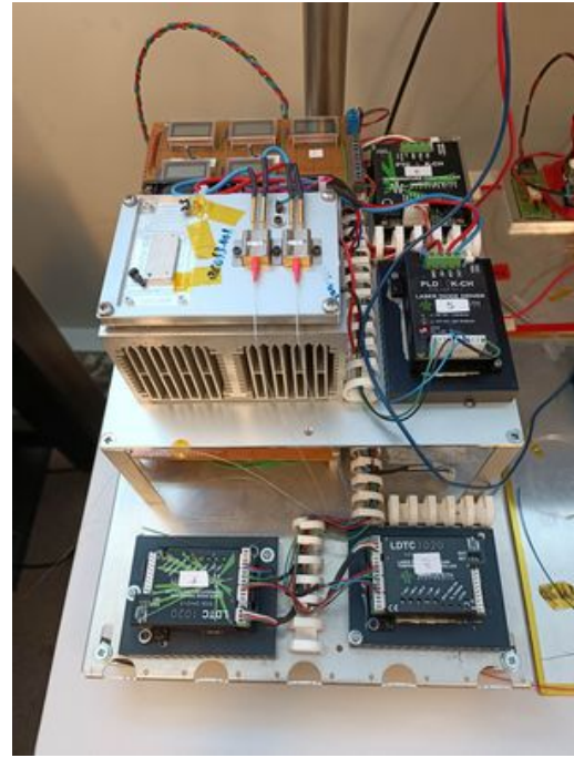
Figure 5.43: Picture of the high-power pump diodes station.
