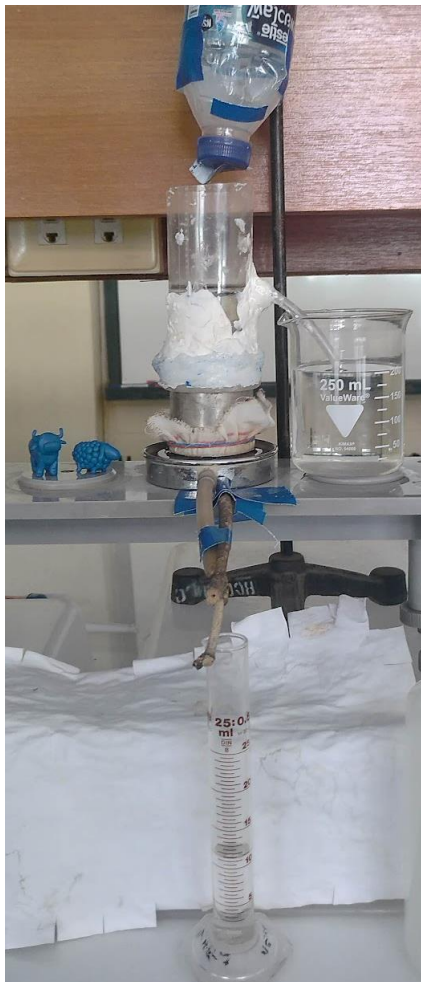
Figure 13 : a) Picture of the home-made constant-head permeameter ; b) scheme of the device
