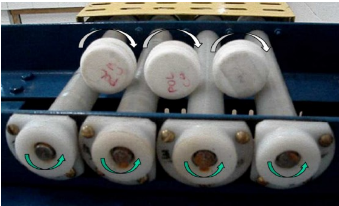
Figure 3 : Device for dynamic curing by rolling of 30 mm diameter moulds (from Kwitko-Ribeiro, 2012)
