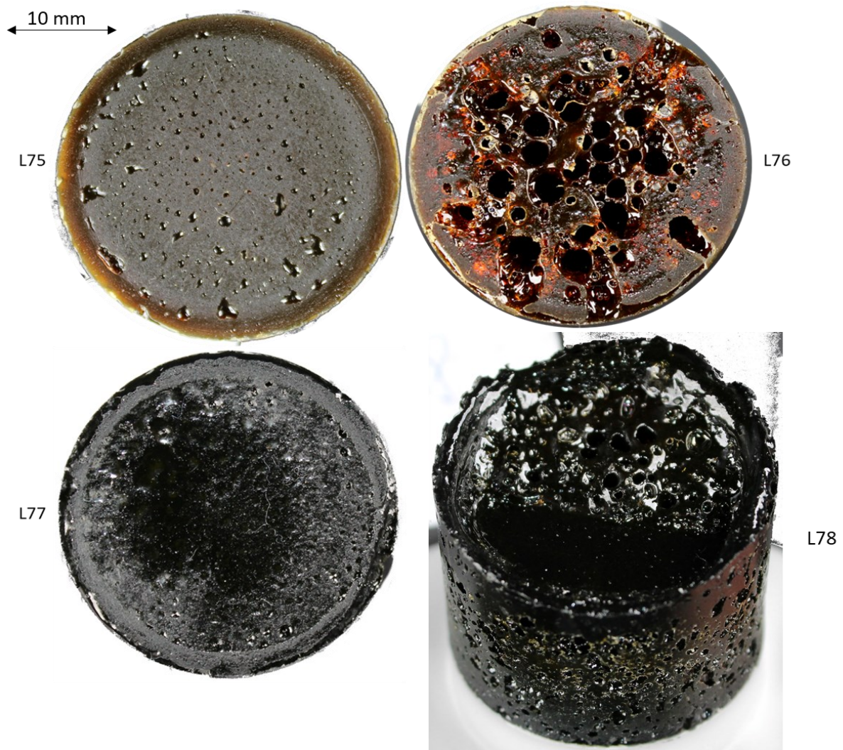
Figure 28: L75 = Struers - iodoform -under pressure; L76 = Struers - iodoform – atmospheric pressure; L77 = Struers - iodoform - 0.1 g BC – under pressure; and L78 = Struers - iodoform - 0.1 g BC - atmospheric pressure
