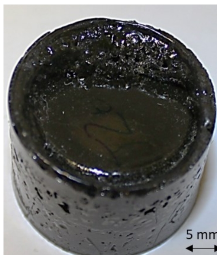
Figure 5: Result of a previous test showing the exothermic reaction that occurred
