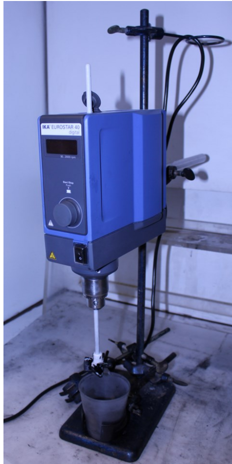
Figure 4: Mechanical stirrer and slightly inclined four-bladed propeller.
