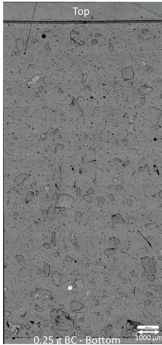
Figure 19 : Vertical section with sample mix (+600/-25 μm) and 0.25 g of BC
