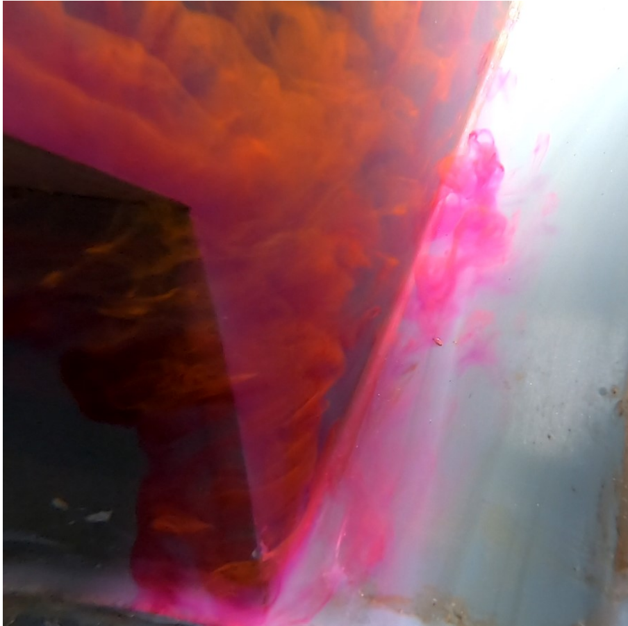
Figure 2.18: Uliège laboratory : inlet flow beneath the upstream overhangs - underwater camera
