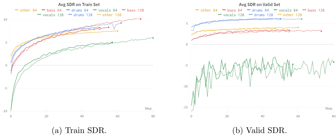
Figure 6.7: Evolution of the Music Demixing Challenge SDR during the training of BSRNN with STDCT. The plain lines depict the models trained with N = 64 while the dashed lines depict the models trained with N = 128 .
