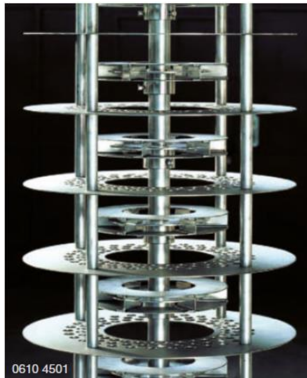
Fig. 2-11: Kühni column internals. (Sulzer, 2018)
