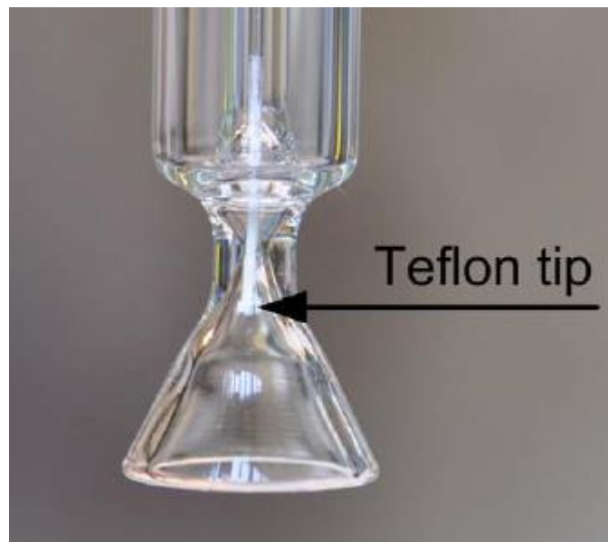
Fig. 5-1: Teflon tip placed in the inlet section of the glass capillary on the sampling cone.
