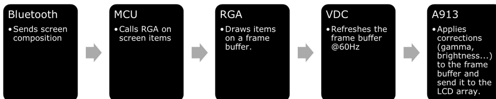
Figure 3.2: From Bluetooth to LCD: The screen composition data flow
