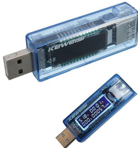
Figure 3.5: The USB ammeter used to evaluate the power consumption.
